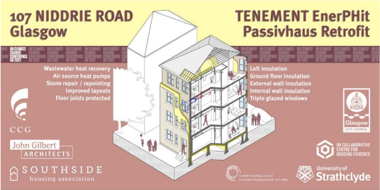
Figure 14: Glasgow’s Tenement EnerPHit Passivhaus Retrofit project. Source: Glasgow City Council
